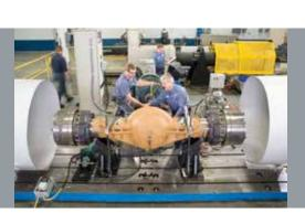
The torsional durability test validates original design calculations and exemplifies the constant pursuit of quality at every stage of systems development.
